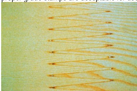
Figure 3: Glued finger-joint
